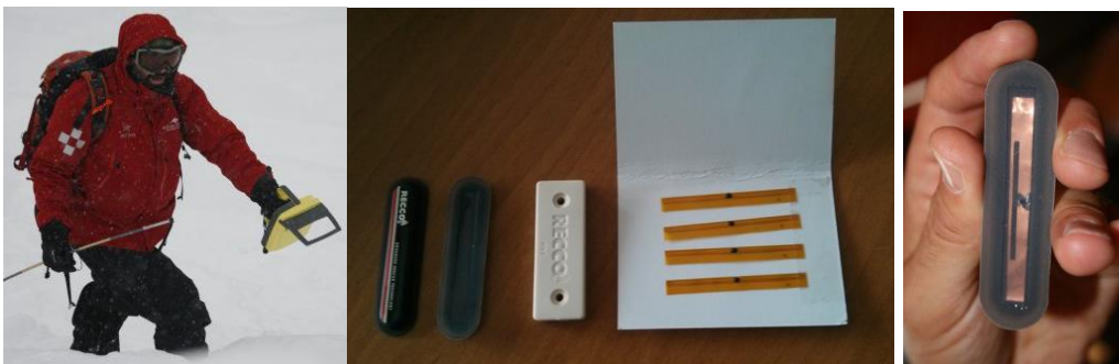
Figure 14: Man equipped with searching antenna and various shapes of R-Fid system
