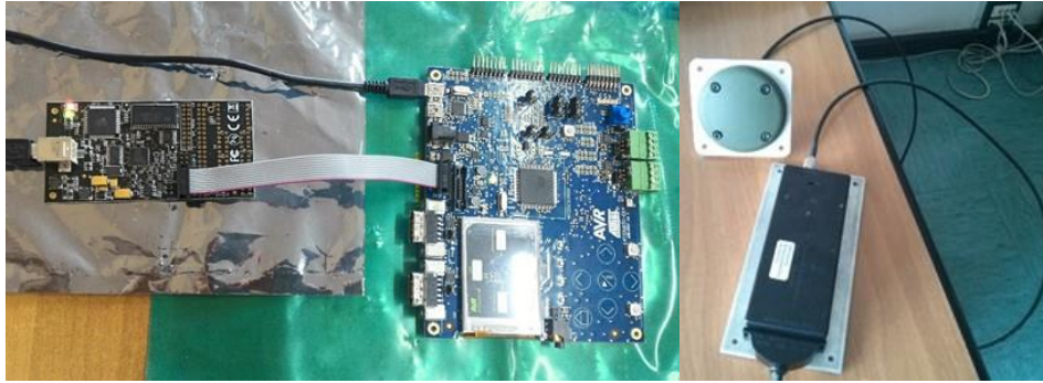
Figure 12: Breadboard fully representative of the flight hardware used for testing and software development.
