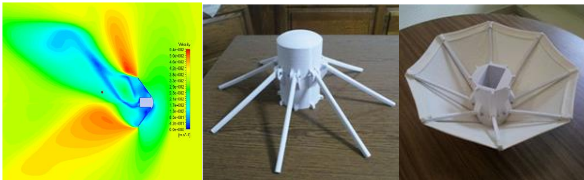
Figure 5: University of Naples activities: CFD analyses. 3D printed model used for drop tests.
