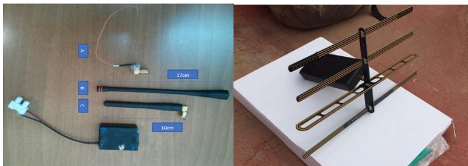
Figure 13: Beacon transmitter components and receiving antenna.
