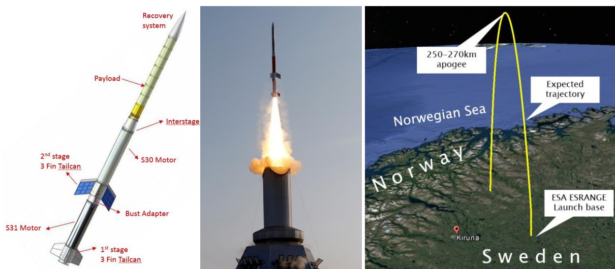
Figure 6: From left to right: The VSB30 Rocket; a launch from ESRANGE base, expected trajectory
